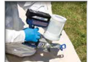
Attach cup with solvent, set to "Clean" and run upside down.
