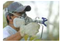
FTx 4-finger gun trigger – full length trigger is easier to hold in continuous spraying.
