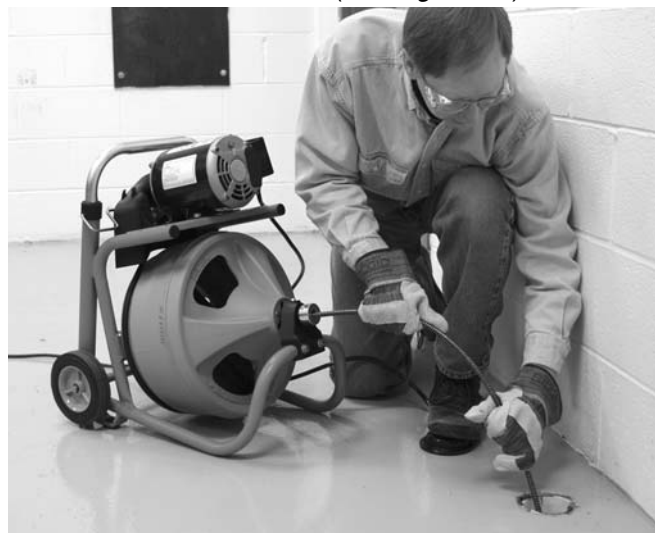
Figure 12 – In Operating Position, Manually Feeding Cable
