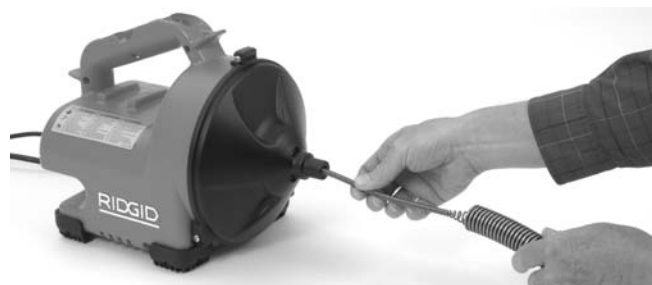
Figure 3 – Feeding Cable into Guide Hose
