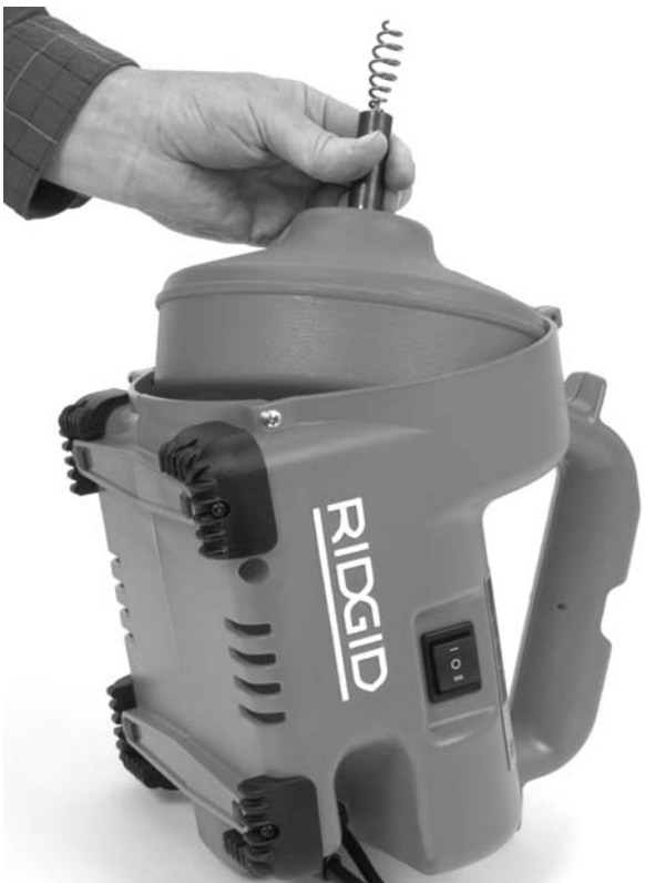
Figure 18 – Inserting Drum Into Machine
