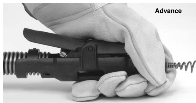
Figure 14A – AUTOFEED in Advance Position
