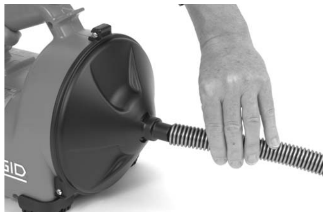
Figure 5 – Attaching Guide Hose to Machine
