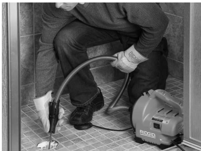
Figure 12 – Using Machine With AUTOFEED
