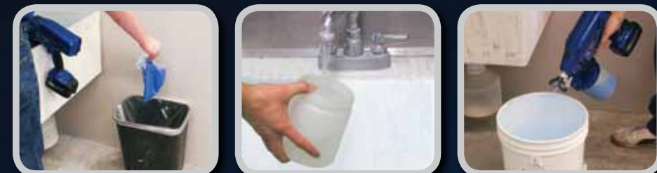
1. Throw away disposable cup liner. 2. Fill cup with water. 3. Reverse the tip and flush.
