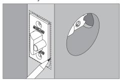
3c Install latch with provided screws.
