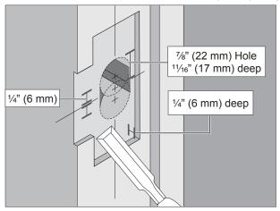
4b Mark and drill 3/16" (4 mm) pilot holes for 3" wood screws.
