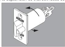
Insert latch into hole. Line up and trace around faceplate.
