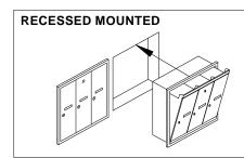
Units fit into a rough opening and are secured with mounting hardware through the back or side panels of the unit. Recessed units include a flanged collar which fits over the rough opening. (Hardware not included.)
