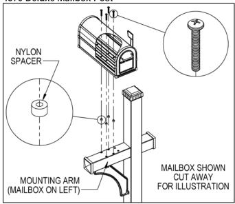
Note: On the 4870 deluxe mailbox post, the longer mounting arm which accommodates the mailbox can be on either the left or right side. When attaching the post to the ground, position the post so the longer mounting arm is on the side desired. Then mount the mailbox on the mounting arm with the mailbox facing the street or roadway.
