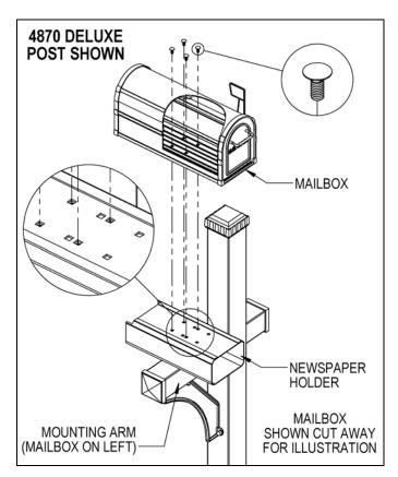
Note: On the 4870 deluxe mailbox post, the longer mounting arm which accommodates the newspaper holder and mailbox can be on either the left or right side. When attaching the post to the ground, position the post so the longer mounting arm is on the side desired. Then mount the newspaper holder and mailbox on the mounting arm with the mailbox facing the street or roadway.
