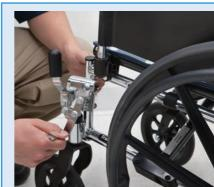
Any wheel lock adjustment should embed the wheel lock shoe at least 1/8" (3/16" for pneumatic tires) into the tire when engaged.
