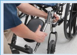
Look for sharp edges on foot-plates and footplate springs. The spring should hold the footplate in any position.
