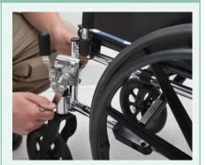
Any wheel lock adjustment should embed the wheel lock shoe at least 1/8" (3/16" for pneumatic tires) into the tire when engaged.
