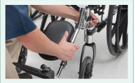
Look for sharp edges on foot-plates and footplate springs. The spring should hold the footplate in any position.
