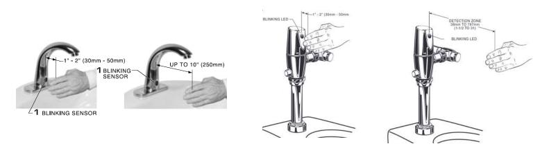
When using the programmer, the sensor will begin blinking for approximately 5 seconds after the "ENTER" key is pressed and the display shows "TRANSMISSION OK".
