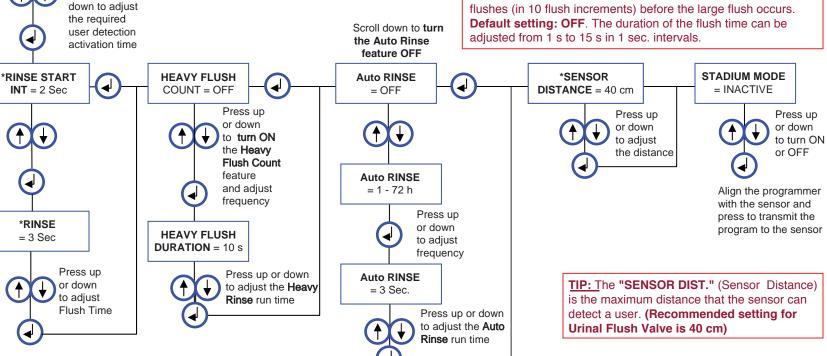
**TIP:** The "Rinse" is the Flush Time (Flush Duration). See Flush Valve Settings Chart
