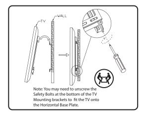
Attach the TV/brackets to the Horizontal Base Plate on the wall, making sure to catch the top claw of the bracket on the rim of the upper base plate. Use the two long safety screws at the bottom of the TV mounting Brackets to tighten the brackets to the base.
