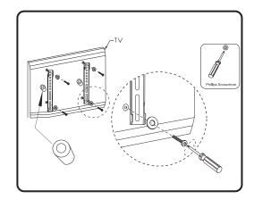
If mounting a Samsung TV with deeper holes, please use **M-D** screws, and Samsung spacers (these spacer are included with Samsung TV).
