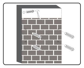
Concrete/Brick wall shown above Use a 3/8" or 10mm drill bit
