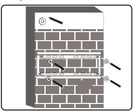
Insert wall anchors into the holes drilled in Step 1, then screw the base plate firmly to the wall with the supplied screws.
