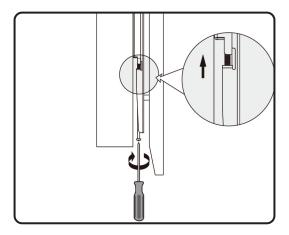
Tighten the two safety screws on the bottom of the bracket until they are **FIRM** against base plate. These screws secure the TV to the base plate and ensure it will not move or shift after installation.
