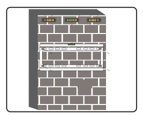
If drilling into drywall, use a stud finder to locate studs. **ONLY DRILL INTO STUDS!!**
