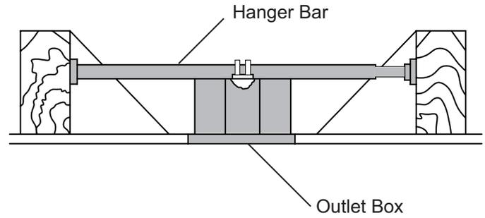
To hang your fan where there is an existing fixture but no ceiling joist, you may need an installation hanger bar as shown above.
