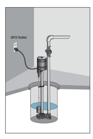
NOTE: The Float Switch comes pre-assembled. Refer to your owner's manual if you need to adjust the ON and OFF position of the float switch.
