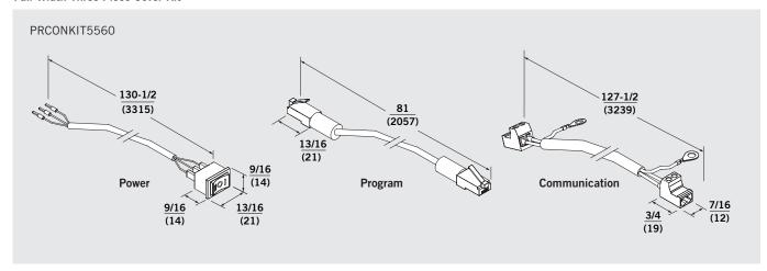
**PRCONKIT5560** — Allows installation and communication of two ED900s on a pair of doors.
