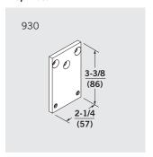
**930** — For mounting arm shoe in top jamb drop application when top door rail is less than 4-5/8" (2" minimum required).
