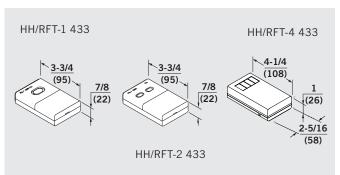
HH/RFT-1 433 MHz (Single Frequency), HH/RFT-2 433 MHz (Dual Frequency), HH/RFT-4 433 MHz (Quad Frequency) — Compact, portable switches. Must be used with RFR receiver. Maximum range is approx. 50 ft (depending on conditions). Works with, or in place of, WS/RFT-1. Powered by 9 V DC battery.
