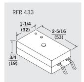
RFR 433 MHz - Radio frequency receiver. Required for use with all DORMA transmitter switches. Powered from the onboard power supply of the ED900. Ideal for applications with range and signal strength problems. Maximum range typically 50 ft (conditions permitting). Surface applies remotely. Operates on 12 or 24 Volts AC or DC. 16 mA nominal (50 mA max. when relay is triggered).
