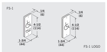
FS-1 — 1-3/4" × 4-1/2" frame plate with a normally open switch. Satin stainless steel frame plate with blue engraving. Frame plate displays the accessibility symbol and "PRESS TO OPEN."
