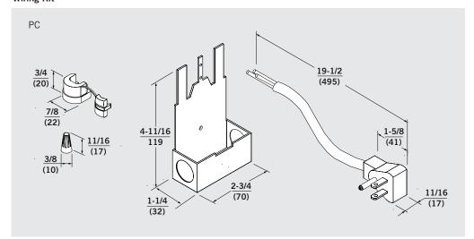
PC — Eliminates need for hard wiring. Permits ED900 to plug directly into 120 VAC/60 Hz receptacle. Cord measures 15" from end cap to center of plug.
