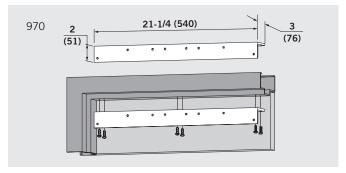
**970** — For mounting ED900 J easily on deep reveal frame conditions or when frame face is less than 1-3/4".
