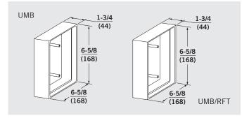
**UMB** — Black ABS universal replacement mounting box for WS-1 type switches.
