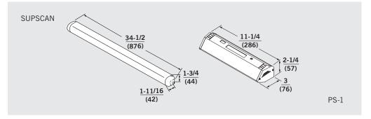
Supscan — Door mounted presence sensor that uses distance measuring technology to project focused active infrared patterns that can be used for safety and reactivation.
