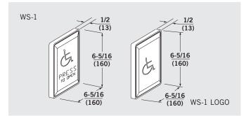
**WS-1** — Tamper-resistant  $6" \times 6"$  wall plate with a normally open switch. Includes a heavy duty injection molded black ABS mounting box. Satin stainless steel wall plate with blue engraving. Wall plate displays the accessibility symbol and "PRESS TO OPEN."
