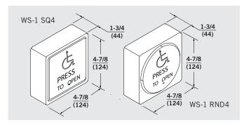
WS-1 SQ4 — Tamper-resistant  $4-1/2" \times 4-1/2"$  wall plate with a normally open switch. Includes a heavy duty injection molded black ABS mounting box. Satin stainless steel wall plate with blue engraving. Wall plate displays the accessibility symbol and "PRESS TO OPEN."
