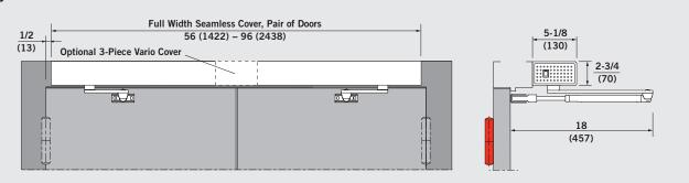
**NOTE:** Refer to the included bumper/stop to limit door travel to a maximum  $110^{\circ}$  to prevent possible damage to the ED900 arm. Where this is not practical, the ED900 J  $\times$  Drop Mount with a surface door stop is recommended.
