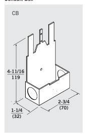
**CB** — UL approved conduit box accessory to provide surface wiring of 120 VAC power to ED900.
