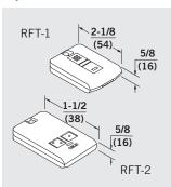
KC/RFT-1 433 MHz (Single Frequency), 800 KC/RFT-2 433 MHz (Dual Frequency) — Similar to HH/RFT-1 or HH/RFT-2, but more compact. Must be used with RFR receiver. RFT-2 requires one RFR per frequency. The small size permits the use as a key chain or in cases where the hand held transmitter is too large. Powered by a watch battery.
