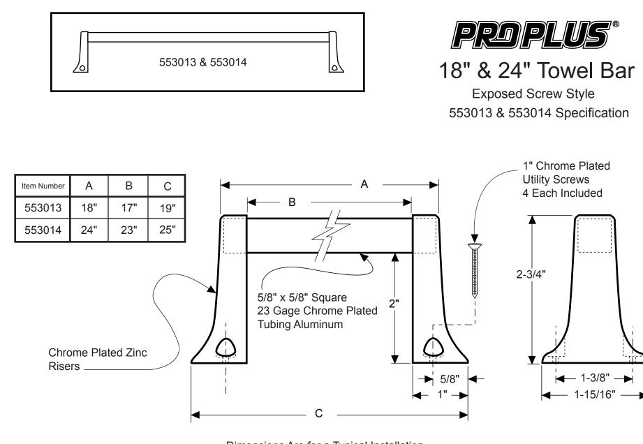
Dimensions Are for a Typical Installation Towel Bar May Be Cut for Custom Installations
