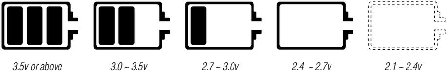
When the battery voltage drops below 2.4 volts, the battery outline will flash and the unit will beep once per minute to alert the low battery condition. When battery voltage falls below 2.1 volts, the shutdown timer is activated. If voltage stays below 2.1 volts for thirty seconds, the DV-41 will beep once and power off. If power is restored during this time, shutdown is canceled.
