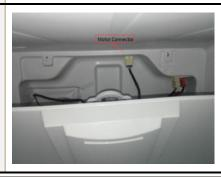
4) Take out the freezing air duct assembly.
