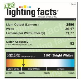
All results are according to IESNA LM-79-2008: Approved Method for the Electrical and Photometric Testing of Solid-State Lighting. The U.S. Department of Energy (DDE) verifies product lest data and results.
