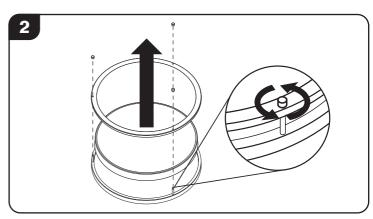
Remove diffuser and decorative ring secured to fixture pan by unscrewing cylindrical post caps.
