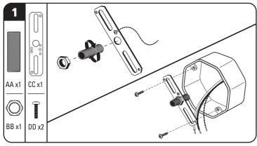
Attach threaded tube (AA) to threaded hole in mounting bracket (CC). Lock in place using hex nut (BB). Threaded tube should extend about an inch beyond wall line. Attach mounting bracket to electrical box using mounting screws (DD) or existing electrical box screws.
