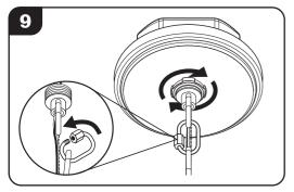
9 Re-attach quick link to the collar mounting stem of the fixture. Raise canopy until collar mounting stem passes through its center and secure by tightening the collar lock ring. Restore power to the fixture.
