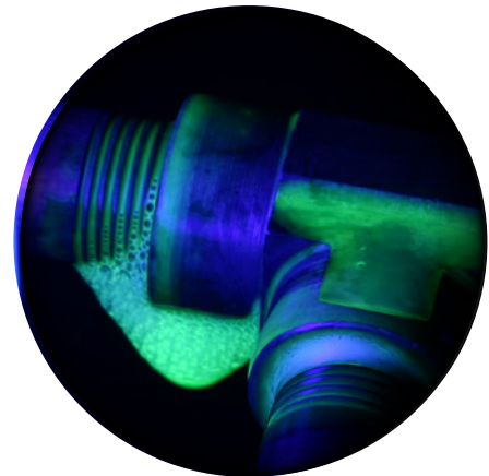
Bubbles detected under Florescent Light
