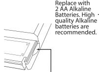
Use the finger bevel on the lower portion of the thermostat to open the easy access battery door.
