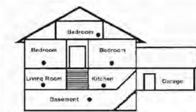
Recommended Alarm Placement for a Multi-Level Residence
