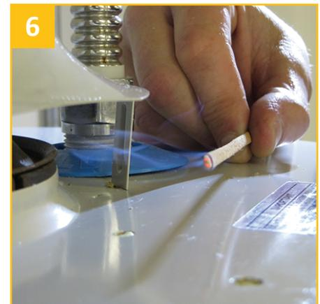
**6 Thermal Switch Tripped (Air Supply Problem)**
