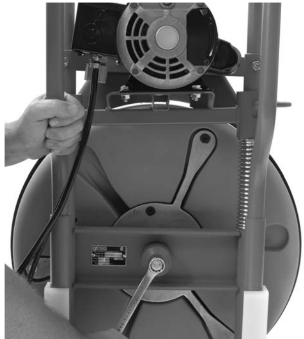
Figure 18 – Removing Drum Bolt
